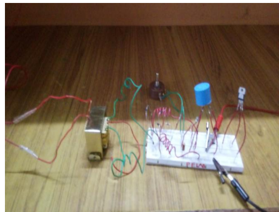
Figure 14 Circuit for firing pulses
