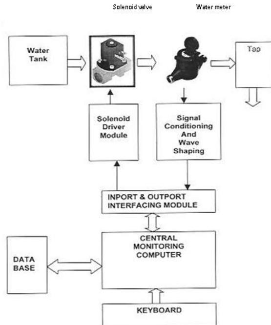
**Fig. 2a: Single Channel Water Metering System**
