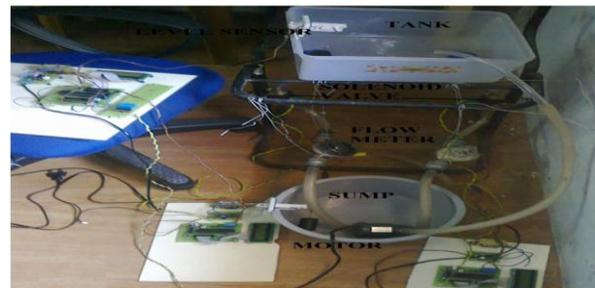
**Fig. 2b: Single Channel Water Metering System**
