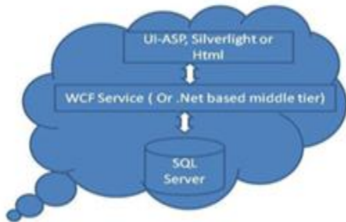
Fig 3:- Application and Database both are on cloud on windows platform
