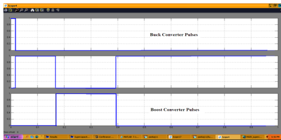
Figure 10: Buck-Boost converter firing pulses in energy discharge mode
